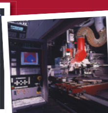
The BIMA machine for fitting hinges onto doors
